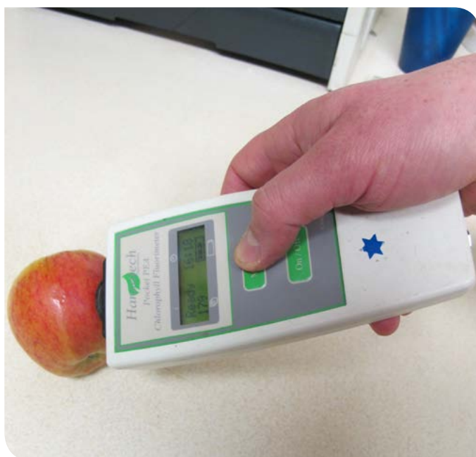
Figure 1: Pocket Pea (Hansatech/Uk) with blue light (wavelength 400 Nm) was used for Gala apple.
